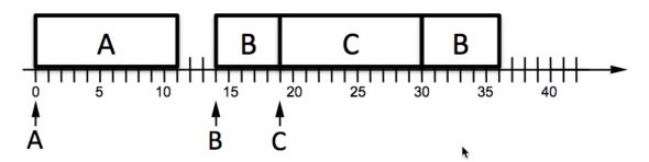
(A) The execution timeline below shows the arrival times of interrupt requests for A, B, and C. Diagram the execution of the A, B, and C handlers assuming a **weak** priority system with the priorities C > B > A. Remember to show the complete execution (all 11 time units) for each handler, labeling each block with the handler that is running.
