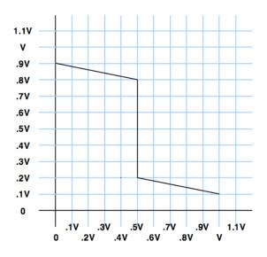
(B) What is the maximum noise immunity that can be realized using this device as an inverter, with an appropriately chosen signaling specification?
