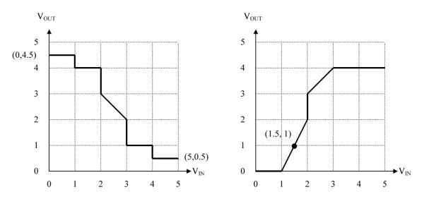
Your job is to choose a single set of signaling thresholds  $V_{\alpha}$ ,  $V_{\mu}$ ,  $V_{\alpha}$ , and  $V_{\mu}$  to be used with both forbidden regions but not pass through those regions. Fill in your answers below, together with the resulting noise margins. You'll get partial credit for anything that works with nonzero noise
