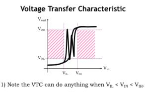
2) Note that the center white region is taller than it is wide ( $V_{OH}$ - $V_{OL}$  >  $V_{IH}$ - $V_{IL}$ ). Net result: combinational devices must have GAIN > 1 and be NONLINEAR.
